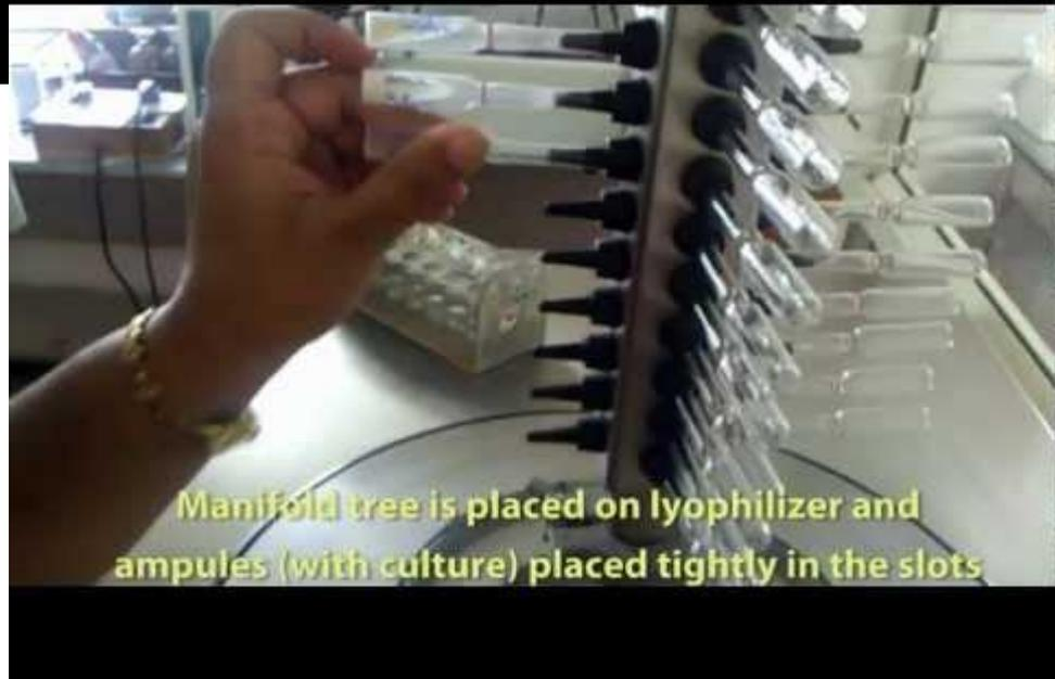
Manifold tree is placed on lyophilizer and ampules (with culture) placed tightly in the slots
