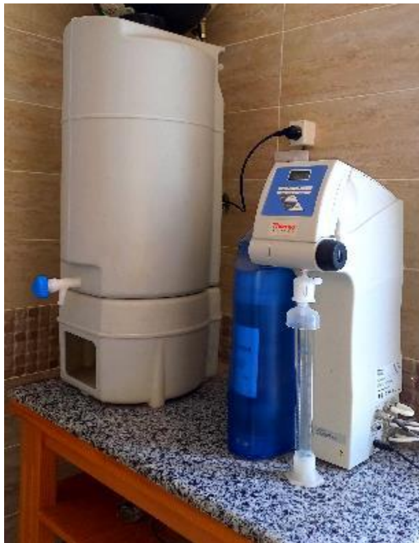
3-17- Water purification system (Therom scientific)
