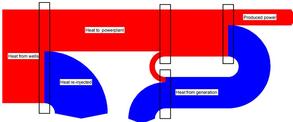
FIGURE 3: Energy streams in a binary power plant
