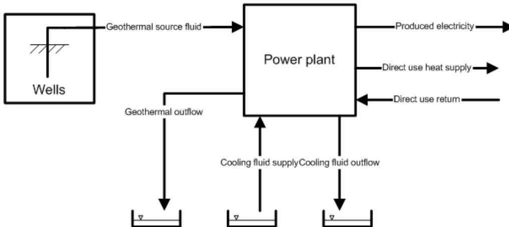
FIGURE 1: Schematic of a geothermal power plant
