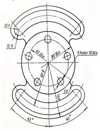
6) Draw the given shape, all dimensions in millimeters.
