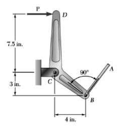
8- Two links AB and DE are connected by a bell crank as shown. Knowing that the tension in link AB is 720 N, determine (a) the tension in link DE, (b) the reaction at C.
