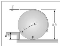
A 500-lb cylindrical tank, 8 ft in diameter, is to be raised over a 2-ft obstruction. A cable is wrapped around the tank and pulled horizontally as shown. Knowing that the corner of the obstruction at A is rough, find the required tension in the cable and the reaction at A.
