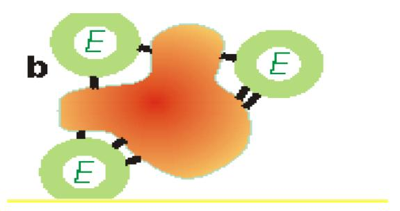
b-Covalent binding : The enzyme (E, greenish) is covalently attached to an insoluble particle (solid porous support) (reddish)
