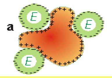
a. Adsorption: The enzyme (E, greenish) is non-covalently adsorbed to an insoluble particle (solid porous support) (reddish)
