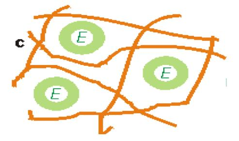
C Entrapment : The enzyme (E, greenish) is entrapped within an insoluble particle porous polymeric matrix (cross-linked polymer, brownish)
