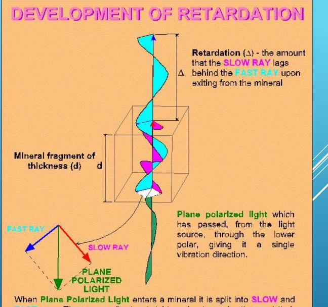
when Plane Polarized Light enters a minaral it is split into SLOW and FLOT rays. These rays vibrate at right angles to each other and their total energy is equal to the energy of the incident ray. Both rays travel through the mineral, with the EACT PLAY exiting the mineral before the SLOW RAY.
